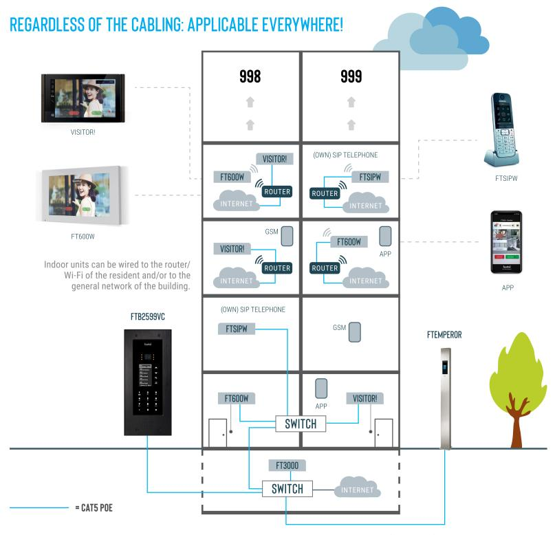
Connect outdoor station + FT3000 Smart SIP Server (if with video) or Fasttel VOIP telephone line (without video) to the internet.
